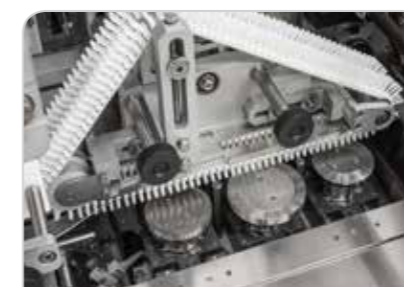
Pusher type infeed conveyor
