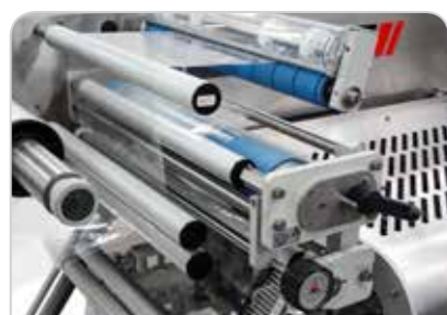
Reel holder with motorised film unwinding
