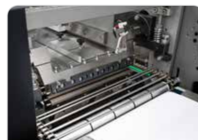
Motorized rollers and convex seal jaws
